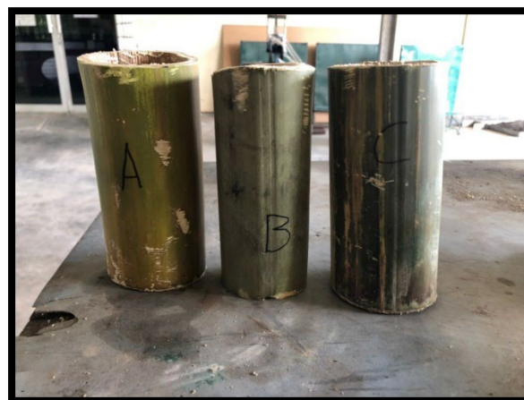
Figure 2: 3 samples of bamboo for compressive strength test
