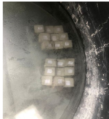
Figure 2: Curing of cube specimens in water
