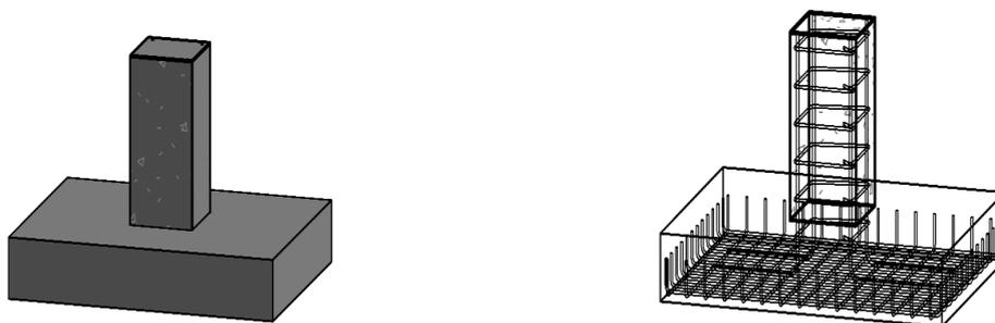
Structural Element without Rebar
