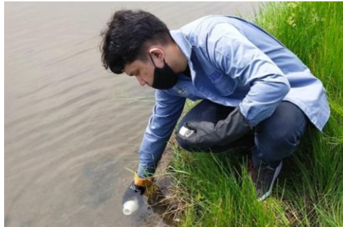
Figure 1: The sampling of water using HDPE bottles
