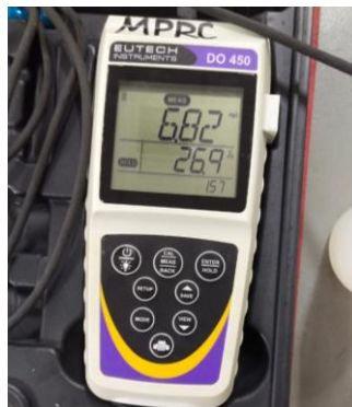
Figure 3: Reading the dissolved oxygen using DO 450 meter
