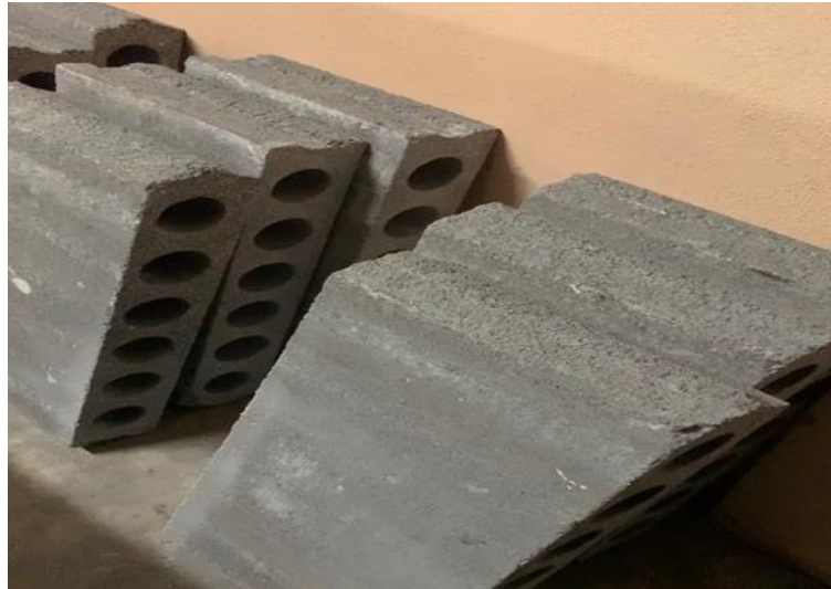
Figure 1: HCWP Samples with Dimension of 300 mm x 600 mm x 100 mm
