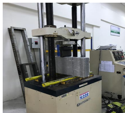
Figure 4: Three-point bending test by UTM machine
