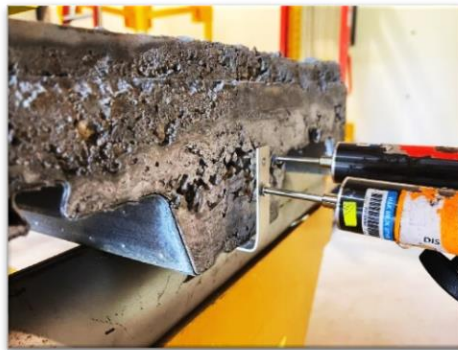
Figure 3: LVDT 2 and LVDT 3 set-up
